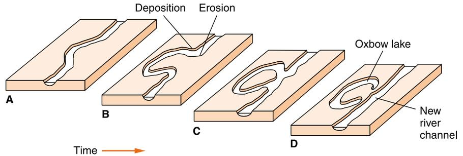
**Figure 12-7** Meanders form where the stream gradient is low and there is a broad floodplain. Diagram A shows the stream starting to form a meander. In B erosion and deposition are starting to cut through the meander. The cutoff is complete in C. Deposition along the edge of the river leaves the meander isolated as an oxbow lake in D.
