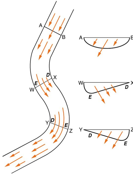
**Figure 12-6** In a straight section of a stream (A–B) the fastest current is at the center of the stream. But in a meander (W–X and Y–Z) the fastest current swings to the outside of the curve. Erosion (E) occurs on the outsides of meanders where the current is fastest and deposition (D) takes place on the inside of meanders where water flows slowest. Erosion and deposition cause streams to change their paths through time.
