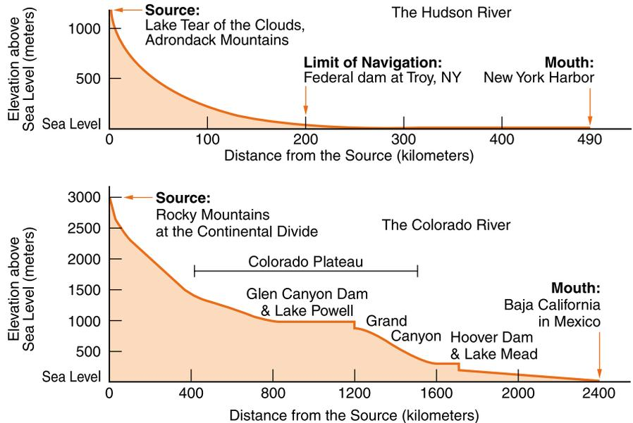
**Figure 12-9** The longitudinal profiles of both rivers are concave as their slope decreases downstream. The double concave shape of the Colorado River profile is evidence of uplift of the Colorado Plateau.
